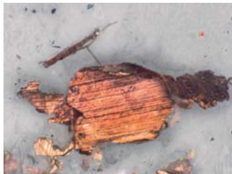
◀ Copper particles, 500 x
